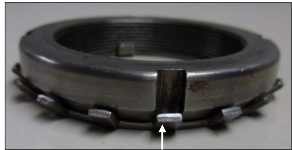
Bend tab up into slot
